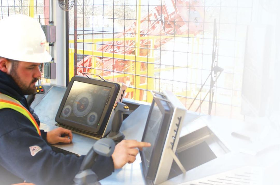
**LOADSAFE® XD** provides class leading automated pipe handling for drill pipe, drill collars and casing. For maximum safety, intuitive joystick controllers are used to lift tubulars from the horizontal position and precisely mate to top drive spindle. Hydraulically powered adjustable holding clamps provide effortless make-up or break-out of tool joints.
